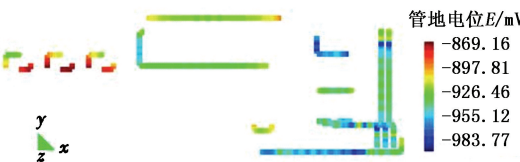
图 9 牺牲阳极进一步加密布置的埋地管网电位分布 Fig. 9 Potential distribution of buried pipeline as sacrificial anodes further encrypting arrangement
