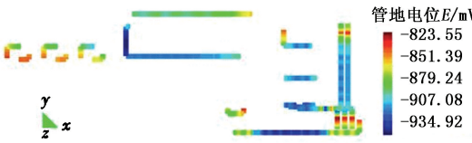
图 7 牺牲阳极加密布置的埋地管网电位分布 Fig. 7 Potential distribution of buried pipeline as sacrificial anodes encrypting arrangement
