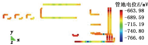
图 5 初步施加牺牲阳极的埋地管网电位分布 Fig. 5 Potential distribution of buried pipeline of applying sacrificial anode preliminary
