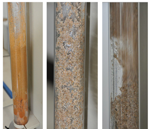
图6 极低水气比条件下的气液固泥状流 Fig.6 Gas-liquid-solid three-phase mud flow under extremely low WGR condition
